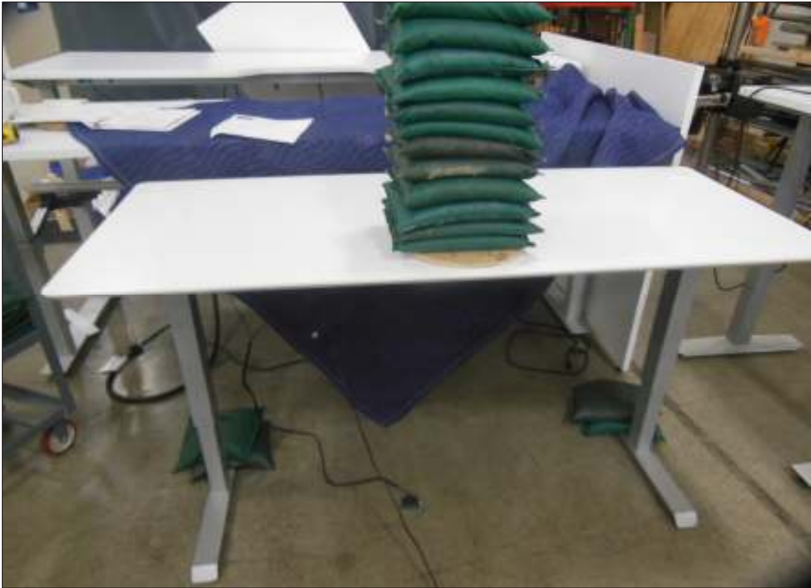
Concentrated Proof Load Test
