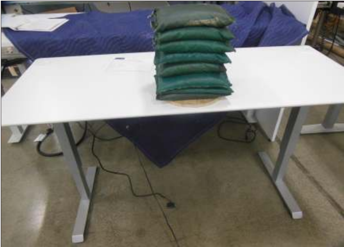
Concentrated Functional Load Test
