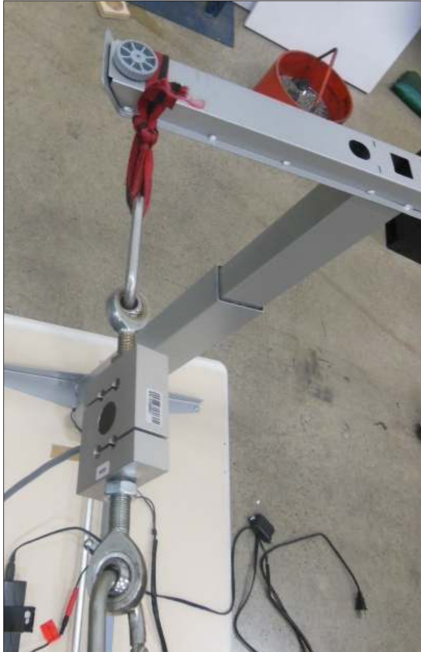
■ Leg Strength Test -- Proof Load
