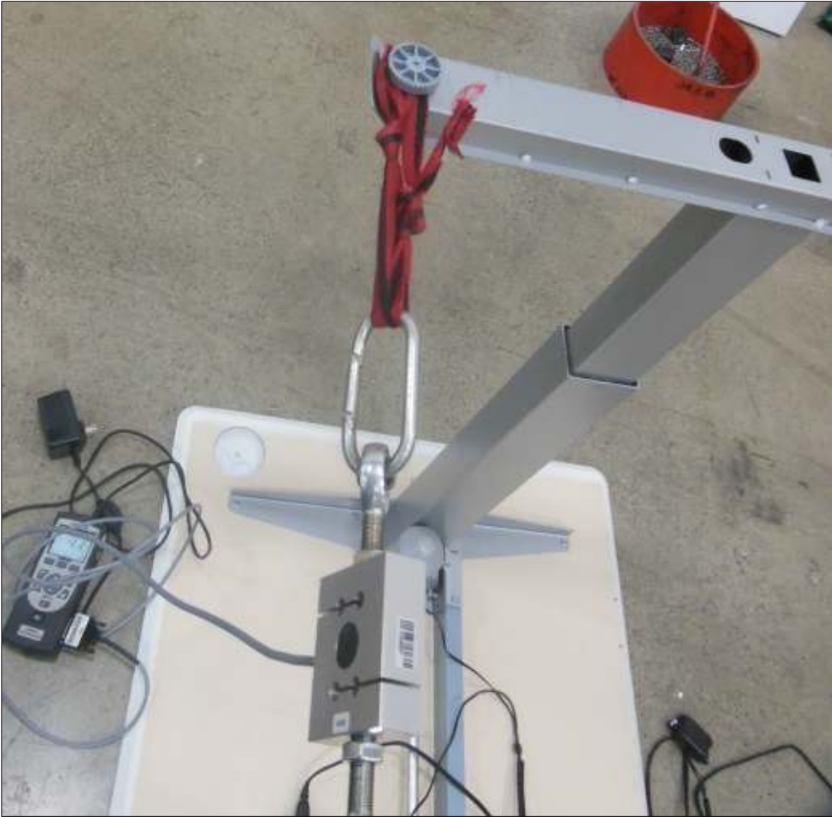
Leg Strength Test – Functional Load
