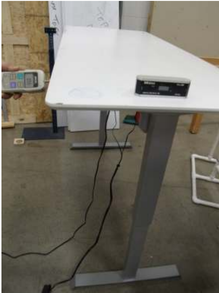
Force Stability Test for Tall Desk/Table Products
