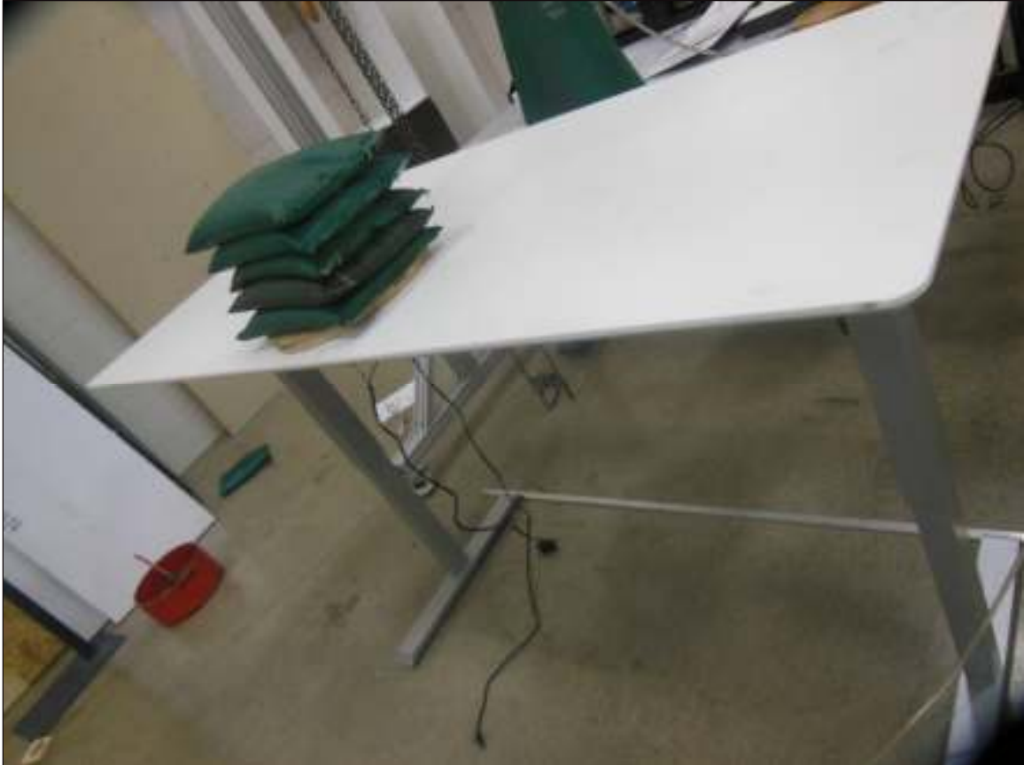
Stability Under Vertical Load Test
