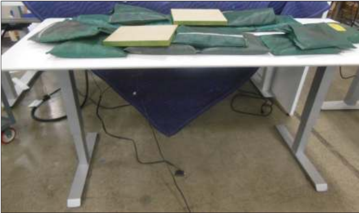
Distributed Functional Load Test
